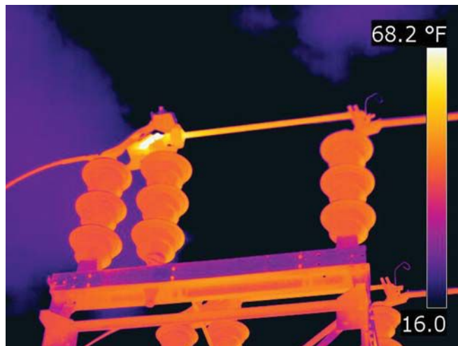
Thermographic image showing a poor connection on a disconnect
