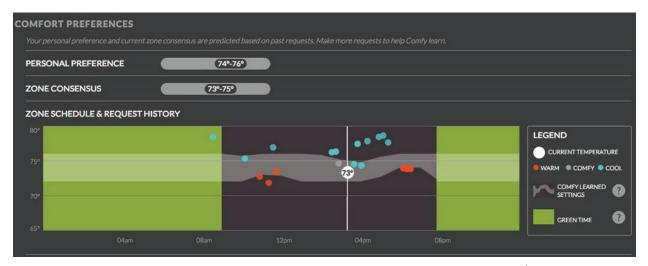
By aggregating data submitted by occupants, a software solution should modify the ongoing temperature setpoints (depicted by light grey band) to satisfy occupant preference first, and energy second.
