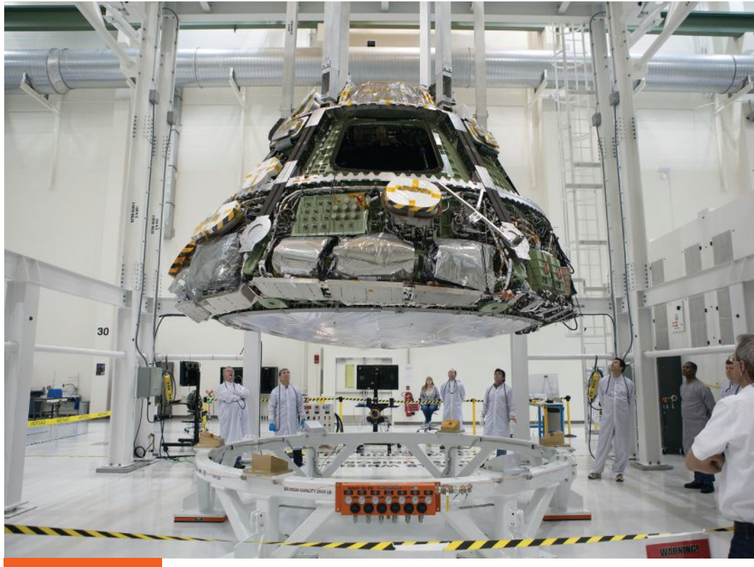
An overhead crane places the Orion module on a work stand, which uses compressed air to "float" the spacecraft through a NASA facility.
