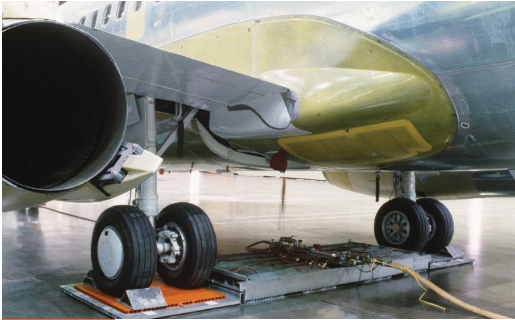
Airplane manufacturing was the first industry to capitalize on air bearings as a flexible and safe load movement method.
