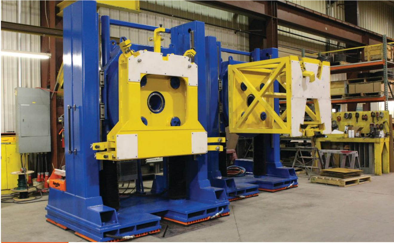
Factory machinery is positioned using air bearings permanently mounted under the structure.
